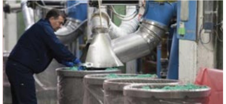
Bata Schindler during the filling of sealing compound
